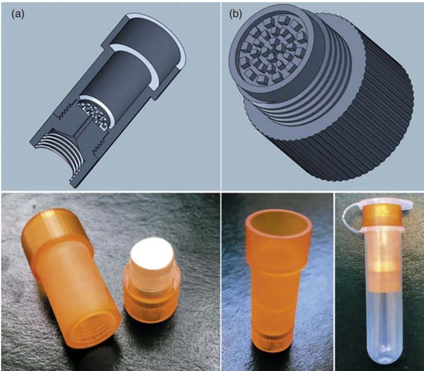
**Figure 34.5** The centrifuge insert design and prototype. Source: Malenfant et al. [22], ELSEVIER.
